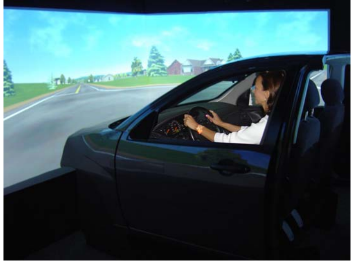
Research-grade driving simulator for the study of the perception and cognition of driving
